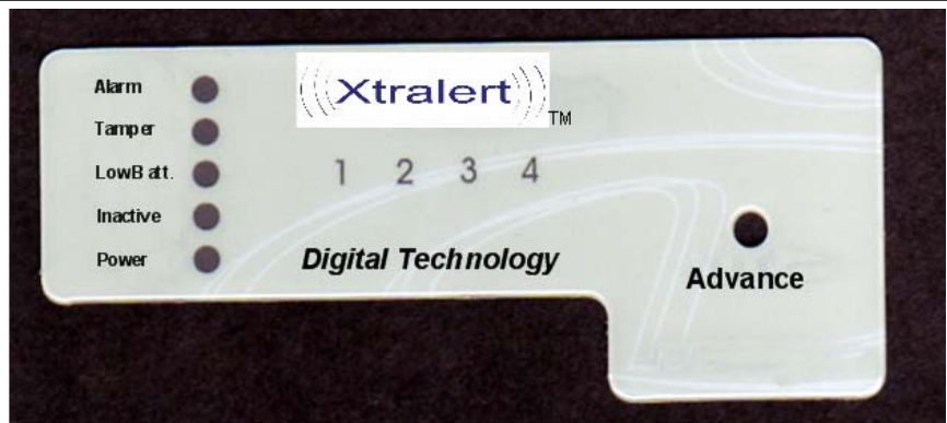
Figure 1: Receiver LEDs and Buttons
