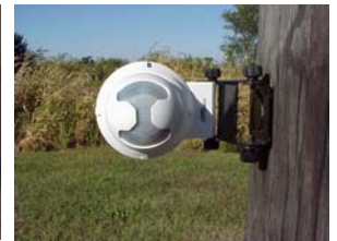
As experimentation, you may want to try rotating the lens assembly so arrows are pointing up and down (vertical) with long range pattern.
