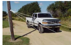
You can also mount the sensor higher to control the length of the beam to a shorter more pinpointed distance.
