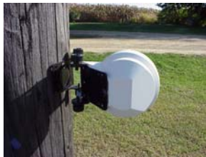
Notice level view of sensor to driveway at about a 3 ft. height mounted behind the pole.
